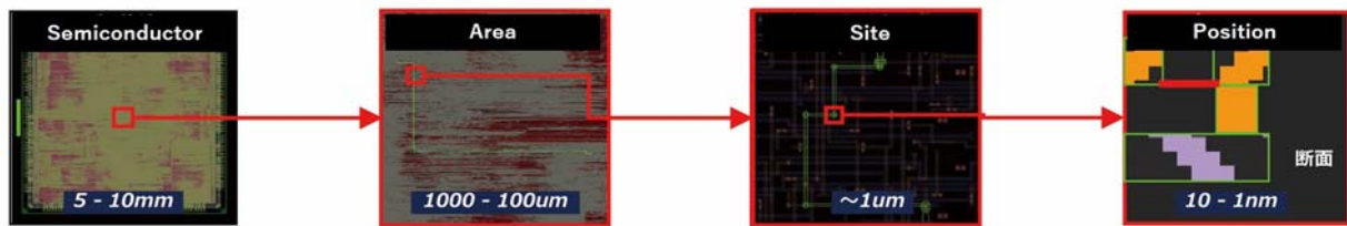
Failure analysis flow
