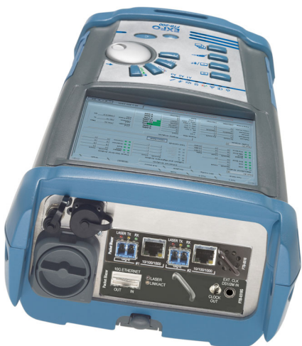
The FTB-8510 Ethernet Test Module can be housed in the FTB-200 Compact Platform. Also shown in the platform, the FTB-8510G 10 Gigabit Ethernet Test Module.
