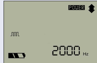
When the test unit finds the correct fiber, an identifier appears on the LCD screen.
