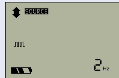
The VFL can be used at either 1 Hz, 2 Hz or in CW.
